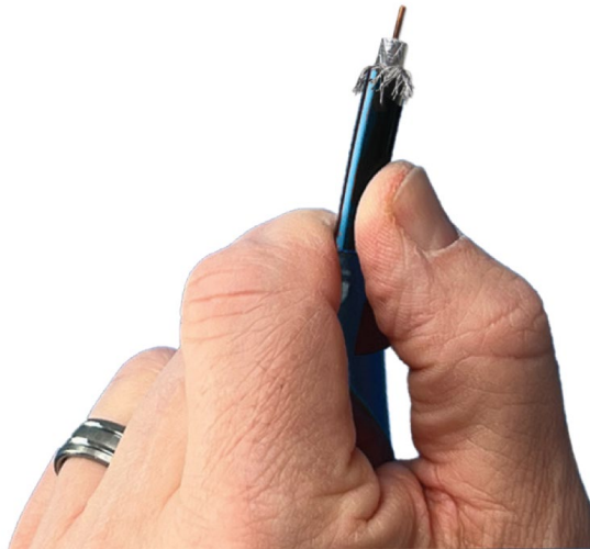
Figure 60: Folding the inner braid against the folded outer braid
