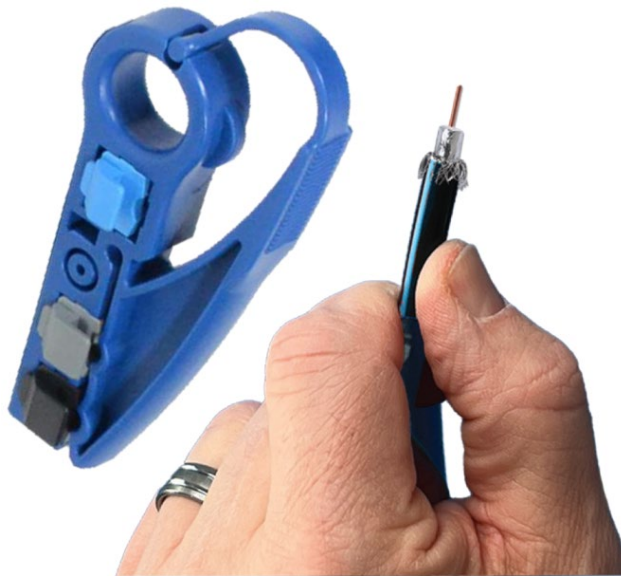
Figure 58: Folding the outer braid against the jacket
