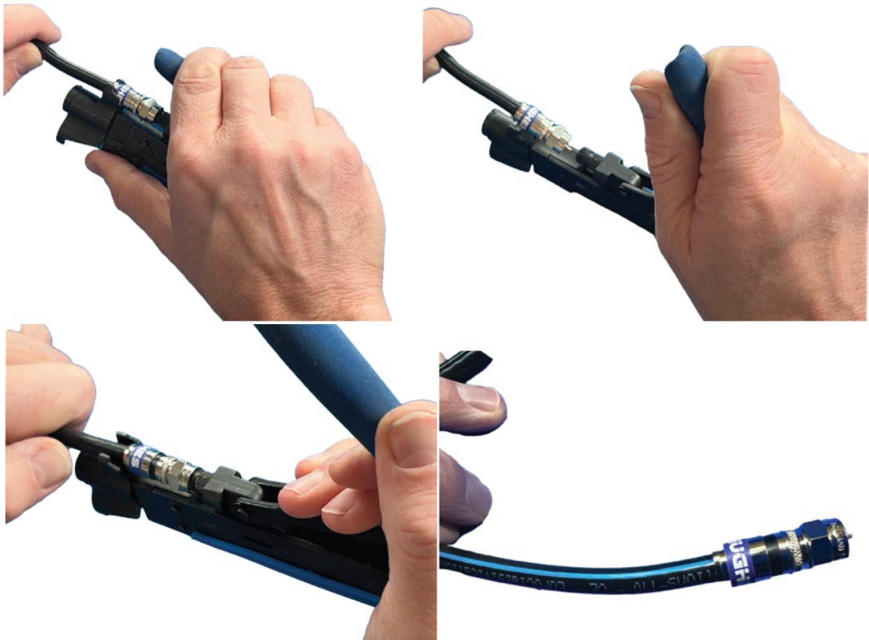
Figure 62: Inserting the IFL cable and connector into the compression tool
